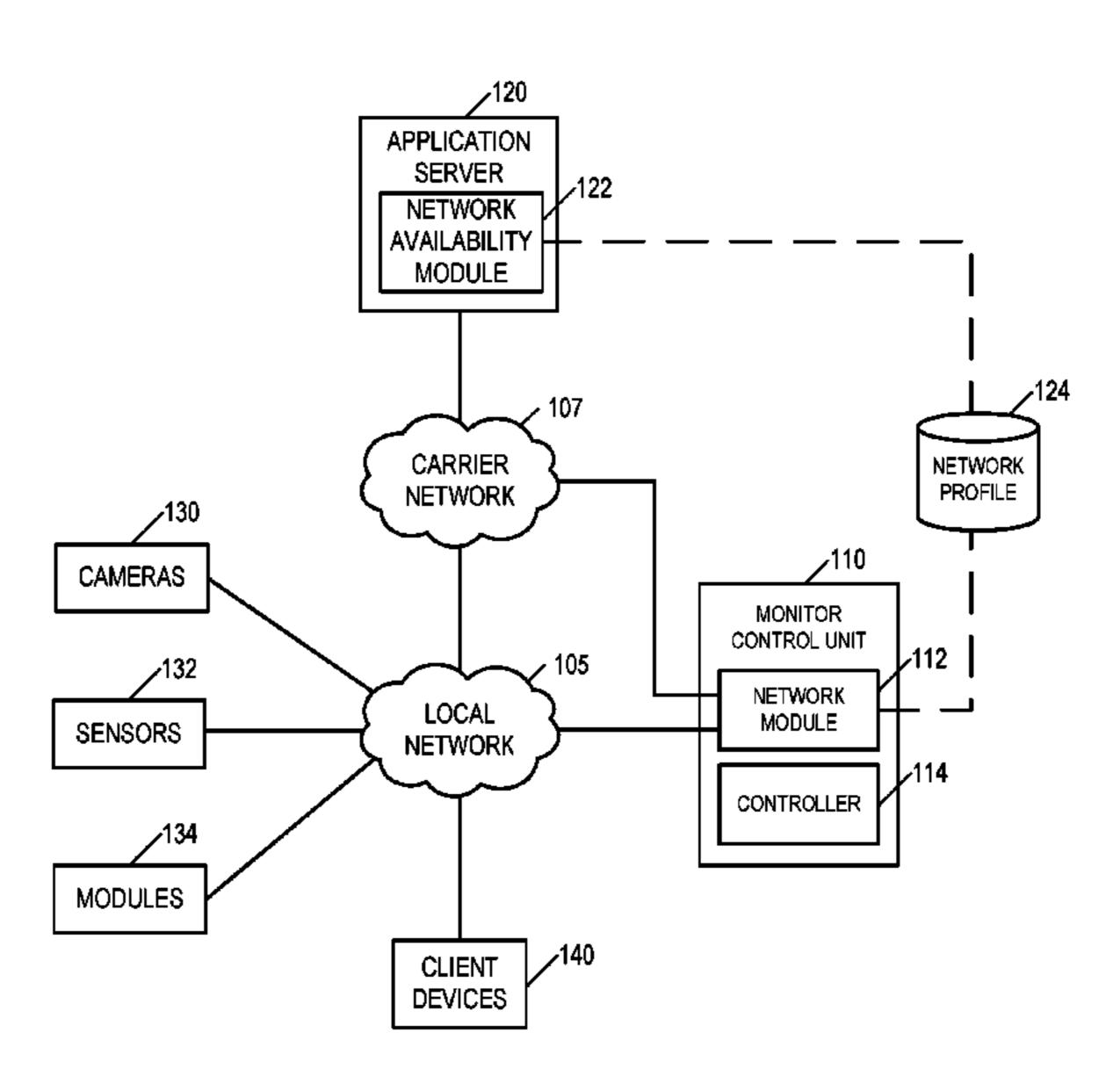
data to the remote server can then be selected from among multiple transmission strategies. The monitoring system data is then transmitted to the server in accordance with the particular transmission strategy.
