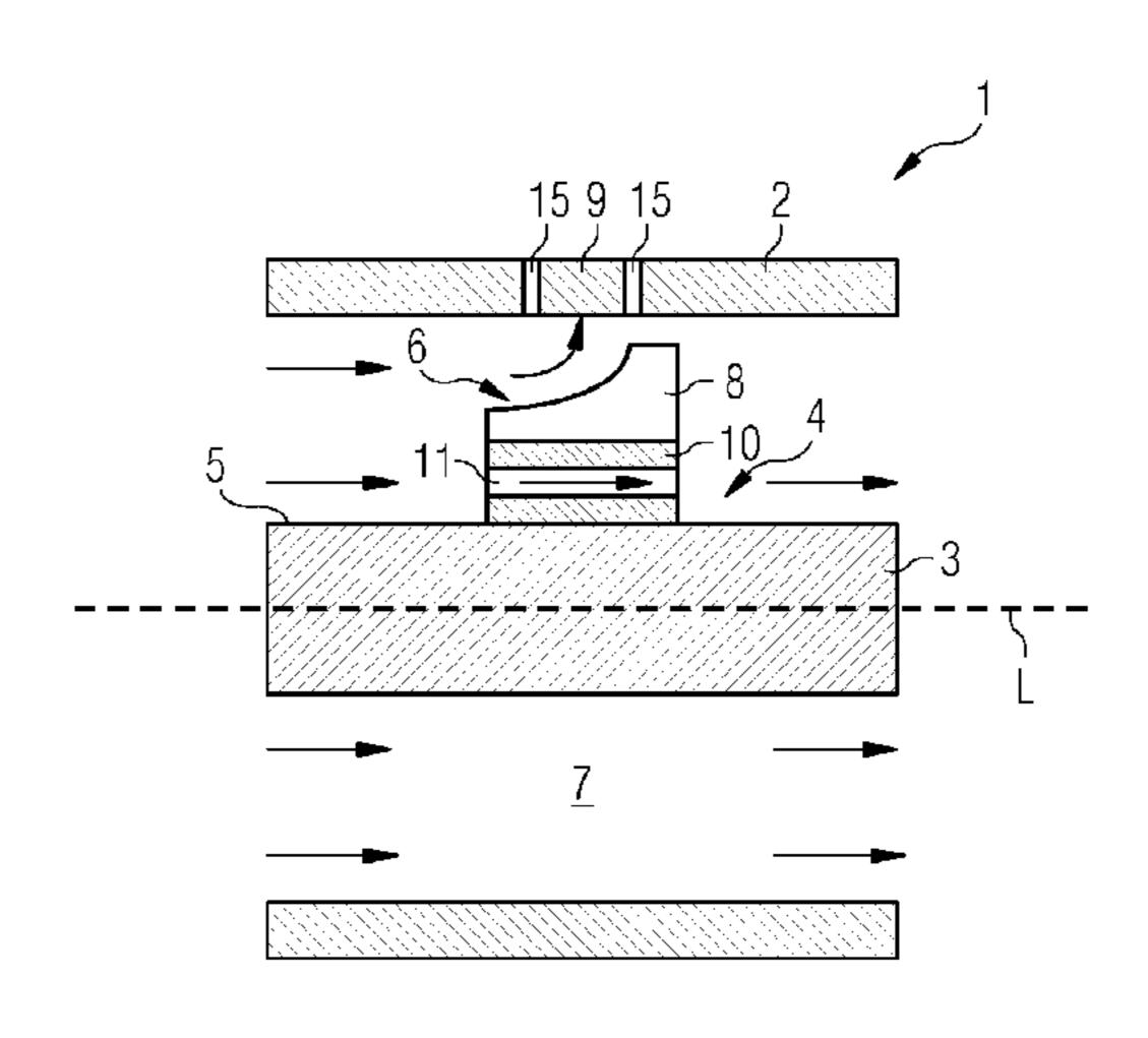
particular of a turbogenerator, wherein at least one blade can be arranged on a prespecifiable section of an outer face of the rotor and in the intermediate space, which blade is designed and can be arranged in such a way that a portion of the cooling fluid flowing in the intermediate space can be radially deflected in the direction of the stator by said blade.
