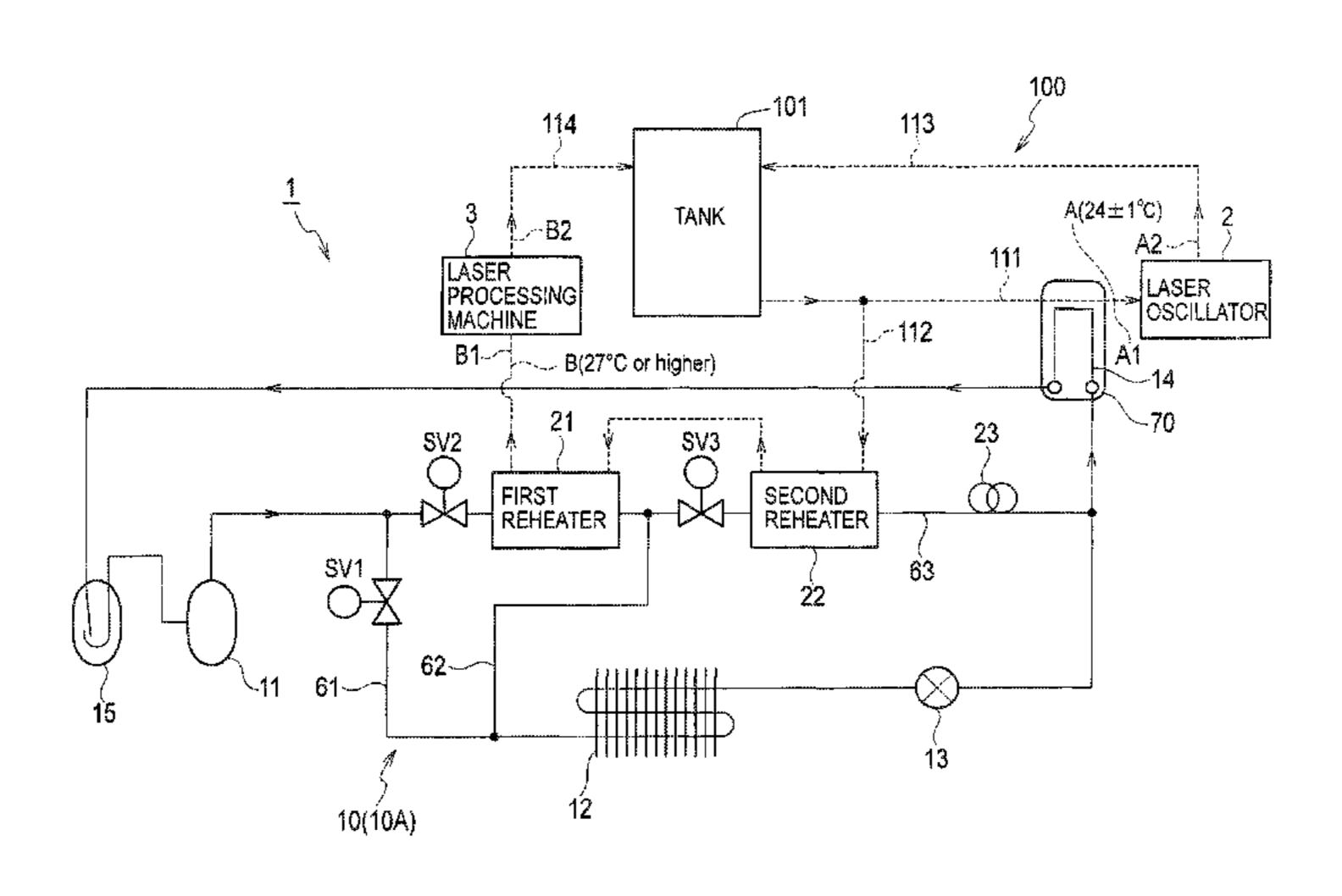
second selective path that supplies the refrigerant to the condenser through the first reheater, and a controller that adjusts quantity of the refrigerant passing through the first and second selective paths.
