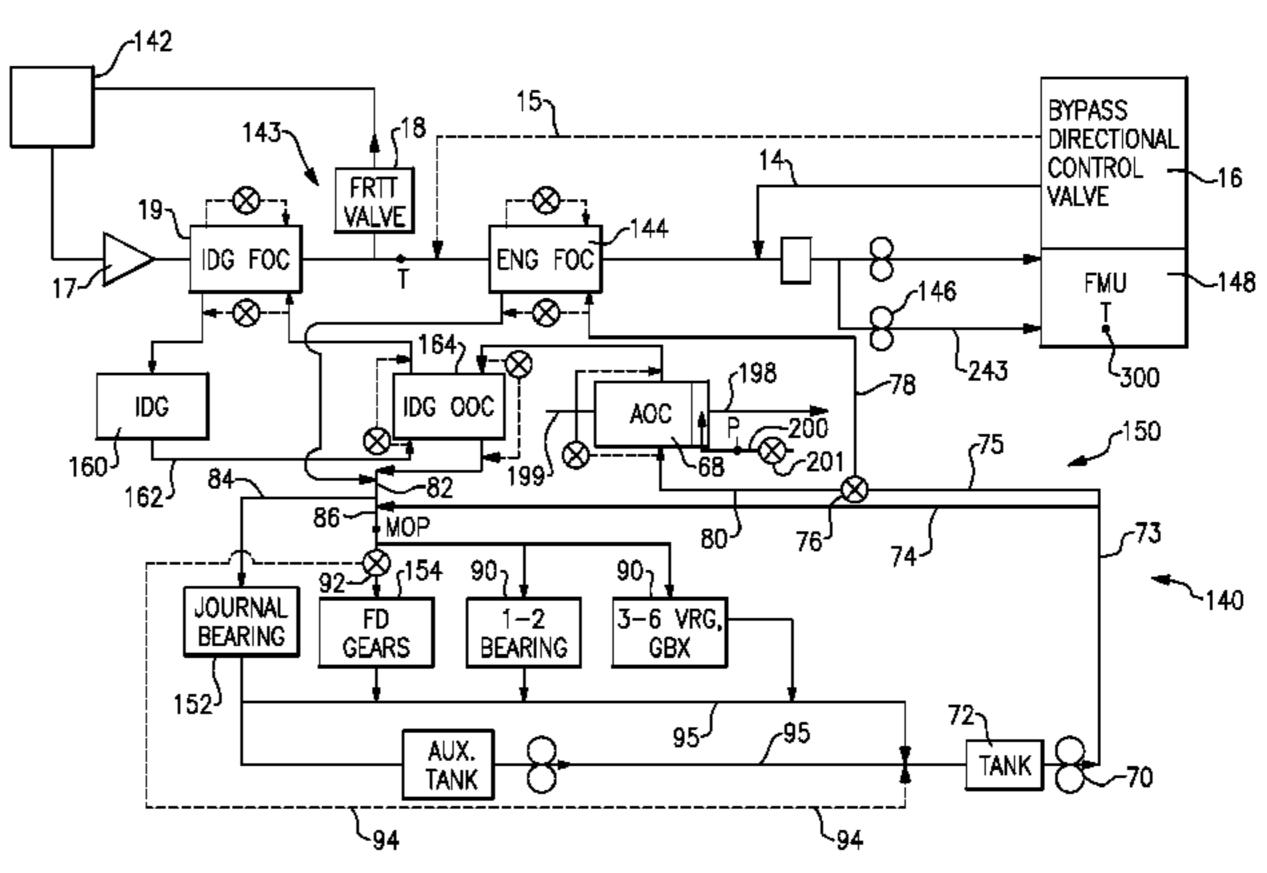
gear system of an associated gas turbine engine. A method and apparatus are disclosed. The heat exchangers include at least an air/oil cooler wherein air is pulled across the air/oil cooler to cool oil. The air/oil cooler is provided with an ejector tapping compressed air from a compressor section to increase airflow across the air/oil cooler.
