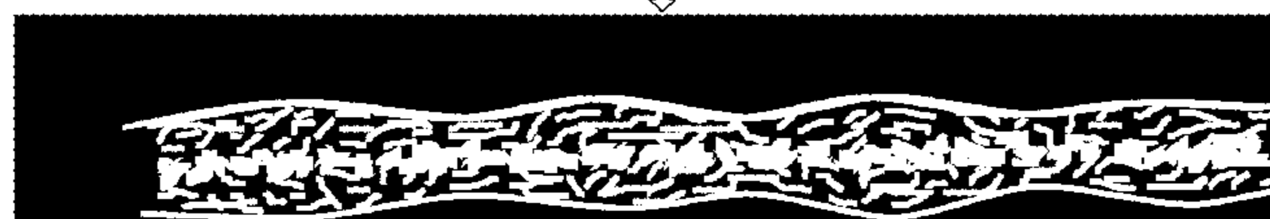
Earlier PVA based yarns -- "hollow from the centre"
