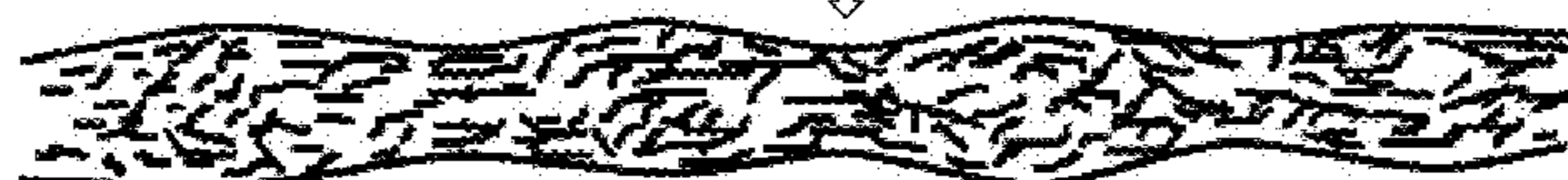
Air Rich yarn -- "homogeneous porous structure"
