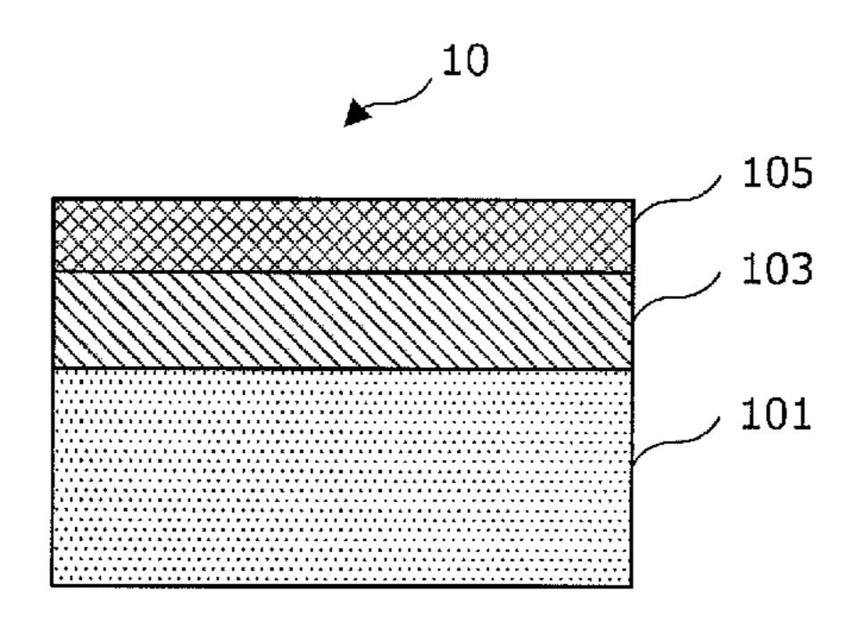
from Mg, Ca, Sr, Li, Na, and K; and a surface coating layer laminated on the Al plating layer and containing at least ZnO.
