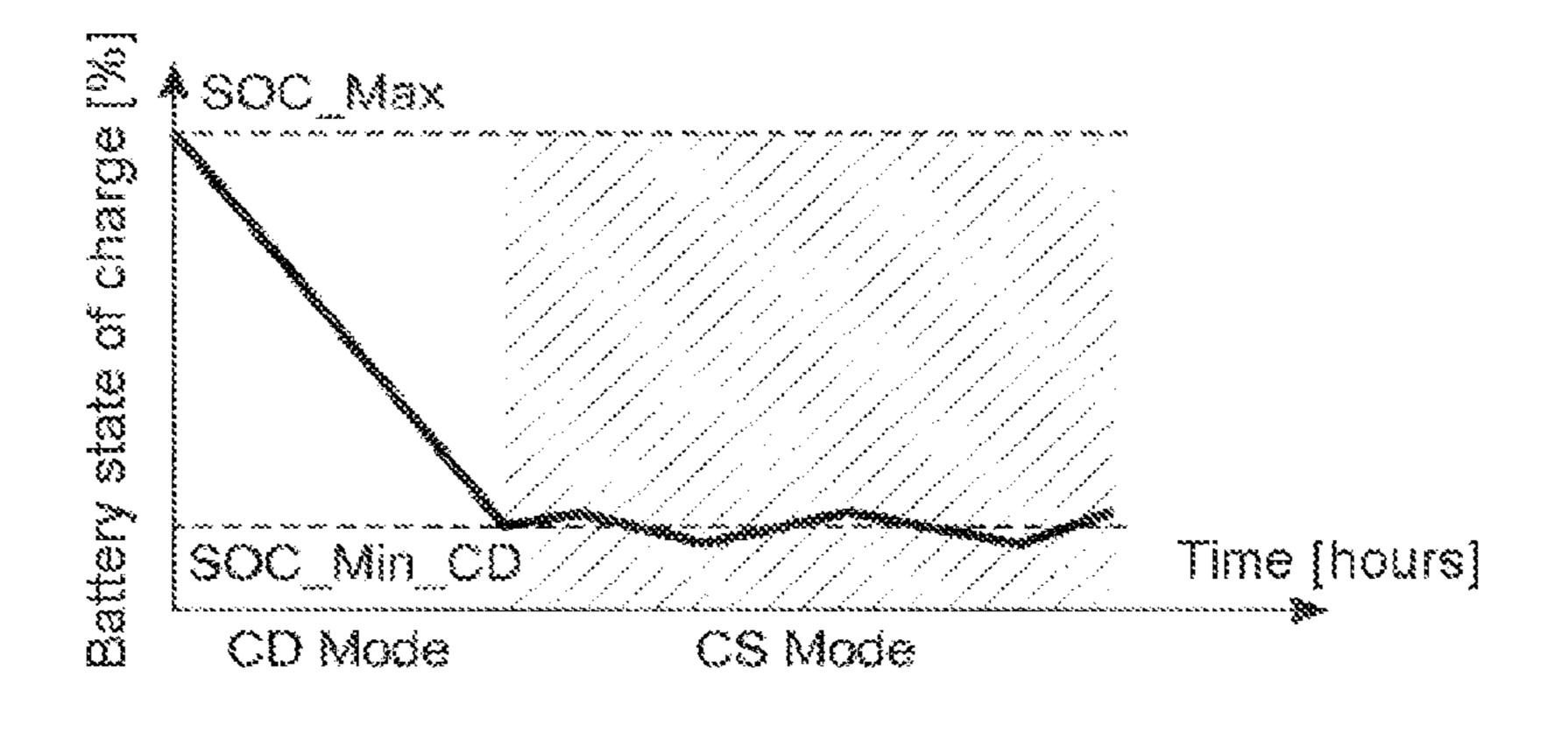
state of charge range linked to the first operating mode when the ageing state of the battery rises above the given ageing state threshold.
