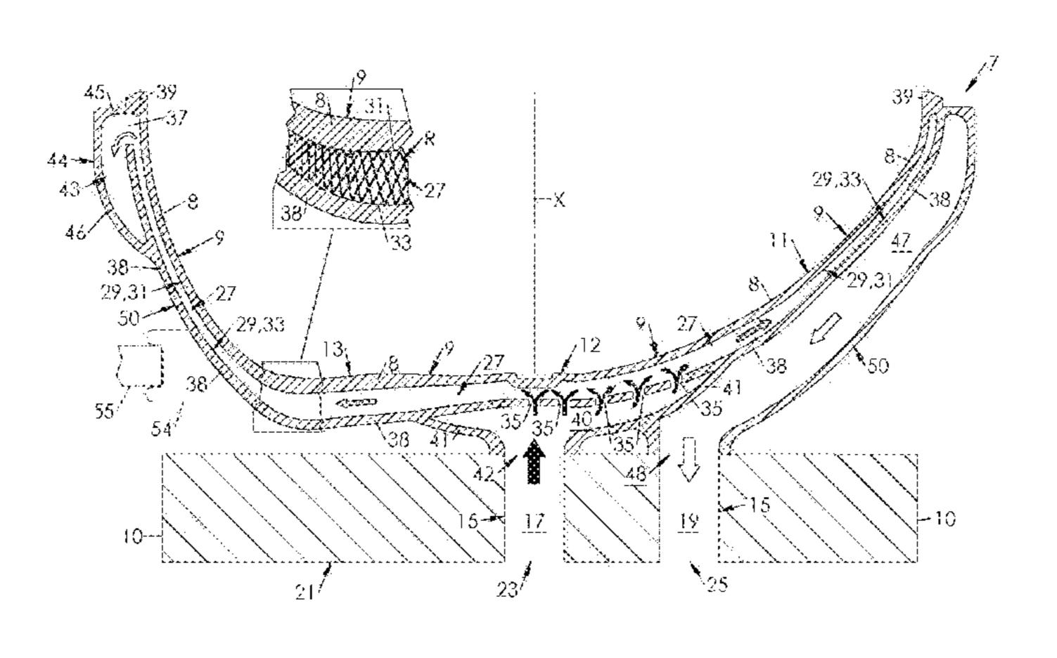
provided with at least one pair of openings (35; 37) leading into the cavity (27) for circulating a heat-transfer fluid inside the cavity.
