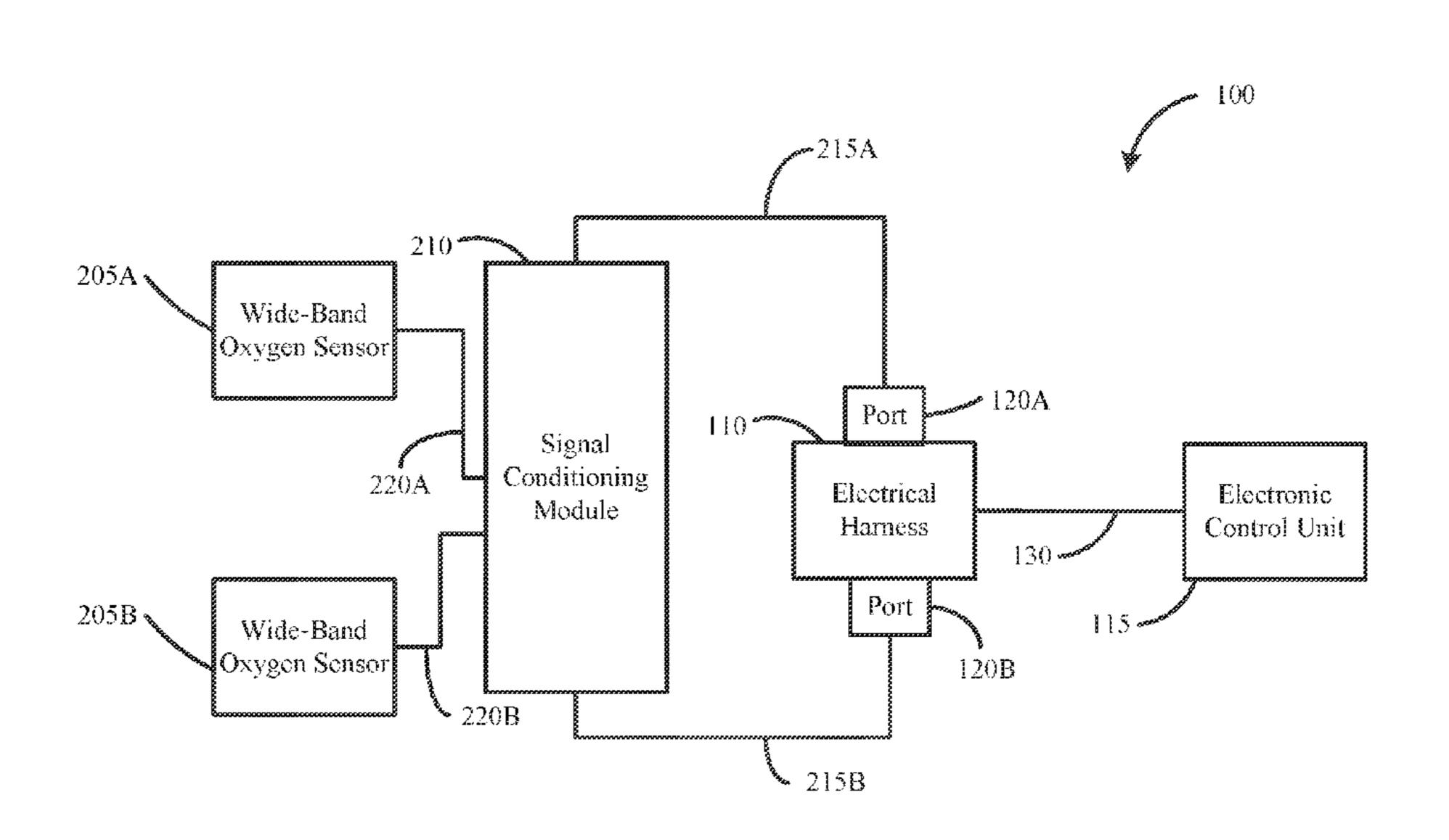
receives first data over the second coupling from the wideband oxygen sensor, converts the first data to second data, and outputs the second data over the first coupling to the electrical harness for transmission to an electronic control unit coupled to the electrical harness.
