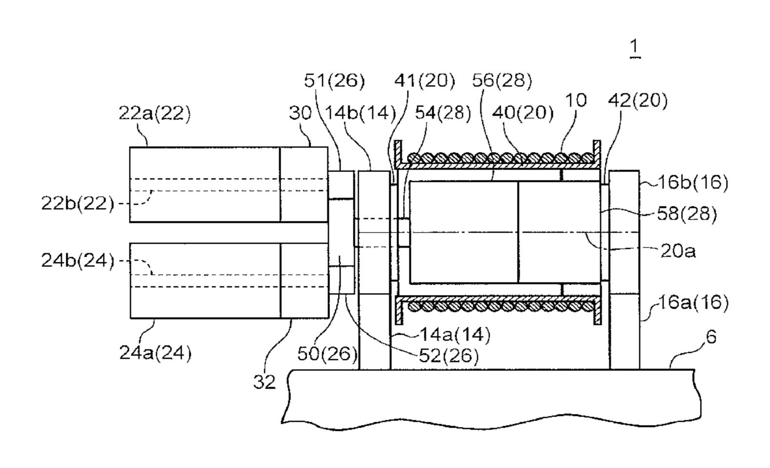
mechanism which combines torques output from the plurality of motors; and a transmitting part which transmits a resultant of torques combined by the gear mechanism to the winch drum to rotate the winch drum to thereby cause the winch drum to wind up or let out the rope.
