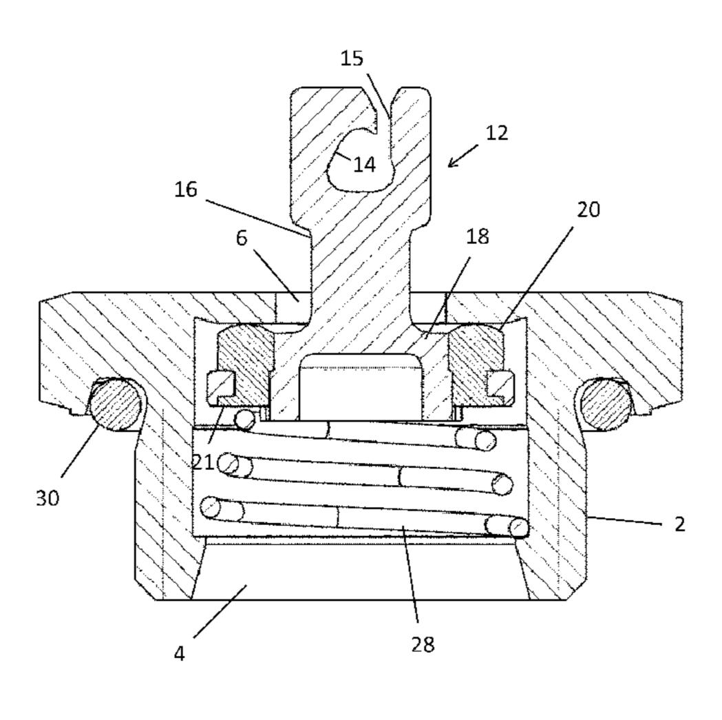
position moved away from the drain aperture. A spring urges the poppet to the closed position. The poppet and the seal are incorporated in a single multi-component injection molded plastic part comprising at least two components. The poppet body is formed of a first plastic component and the seal is formed of a second plastic component partially embedded in the first plastic component.
