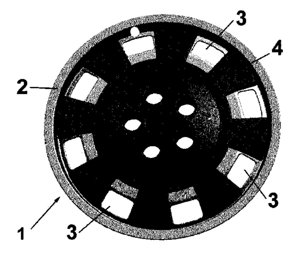
which the holes (3) are completely or partially covered, when the rotating speed of the wheel is higher than a preset speed, and it is characterized in that the cover element (4) is also linked with the base element (2) by a temperature activation element (6), so that when the temperature sensed by said temperature activation element (6) is higher than a preset temperature, the temperature activation element (6) moves the cover element (4) to said rest position.
