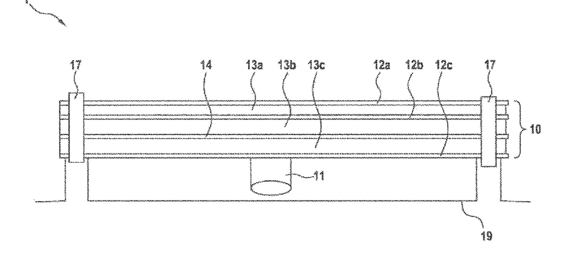
mounted in the vehicle, the circuit board shields the electromagnetic radiation that is emitted by the at least one electrical or electronic component at least with respect to the interior of the vehicle. And to a method for manufacturing such an apparatus.
