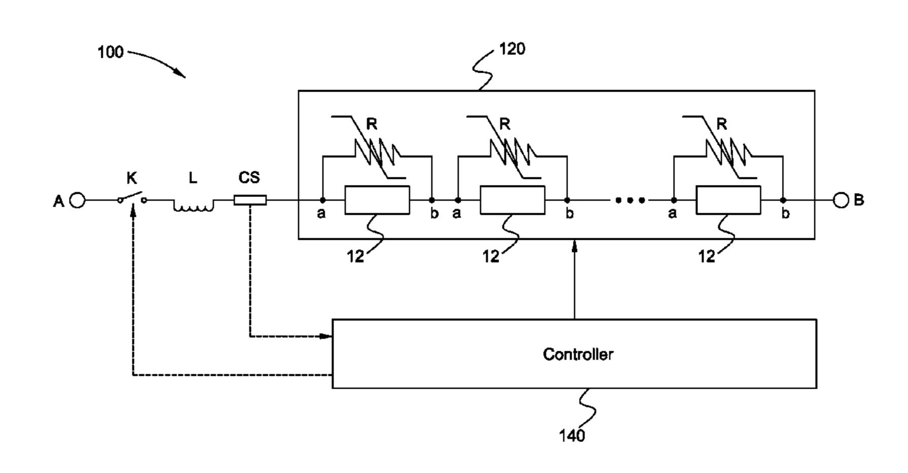
conduction control. The controller controls the multiple switch modules to connect current in the system, and break current of the multiple switch modules according to sensed current signals from the current sensor.
