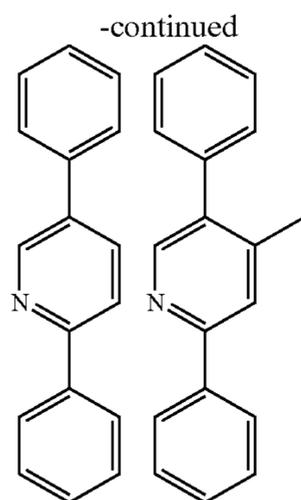
Novel phosphorescent organic materials are provided. The organic materials are compounds containing at least one ligand having an alkyl substituent and an aryl substituent such that the substituent aryl is twisted out of plane (i.e., twisted aryl in this document) more than the usual unsubstituted phenyl-phenyl. The compounds may be advantageously used in organic light emitting devices. In particular, the compounds may be useful as an emitting dopant in such devices.
