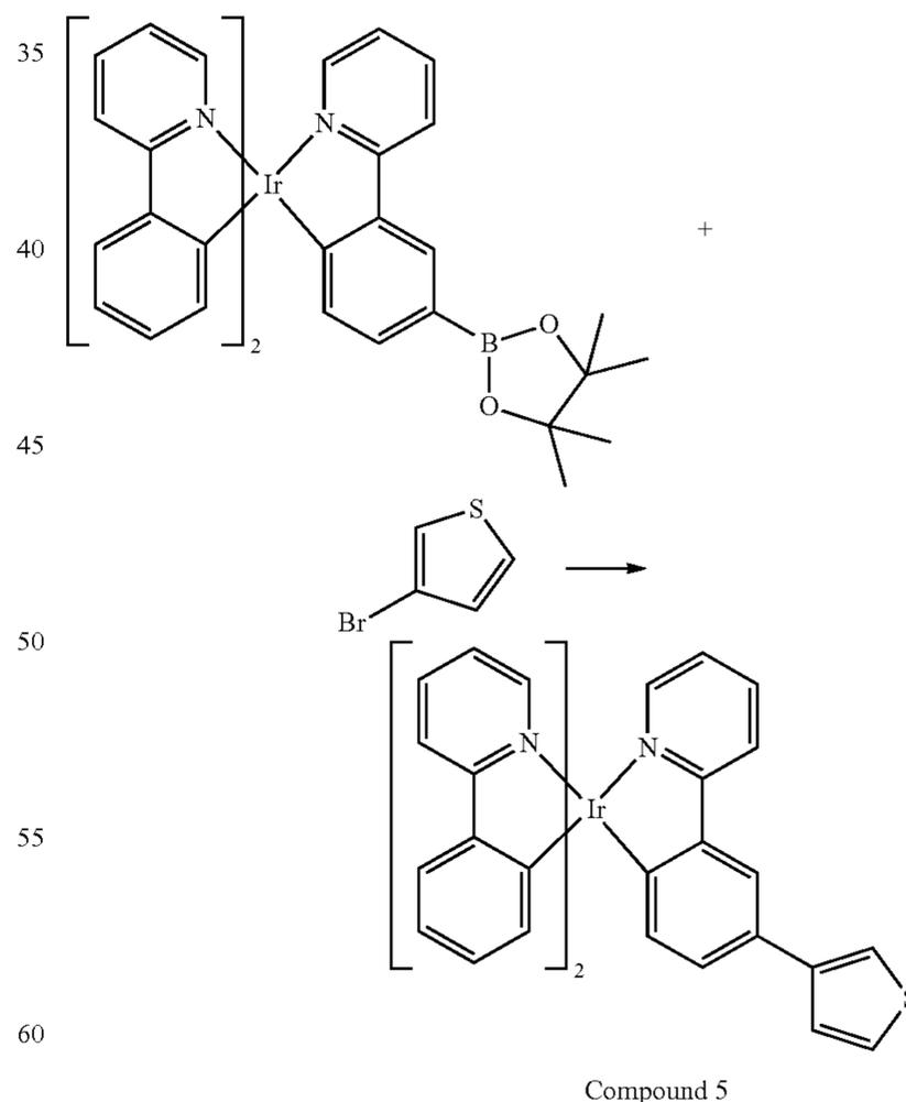
Irppy intermediate (1.50 g, 1.90 mmol), 3-bromothiophene (1.61 g, 9.6 mmol), tris(dibenzylideneacetone)dipalladium(0) [Pd<sub>2</sub>(dba)<sub>3</sub>] (0.02 g, 1 mol %), tricyclohexylphosphine (0.04 g, 4 mol %) and potassium phosphate tribasic
