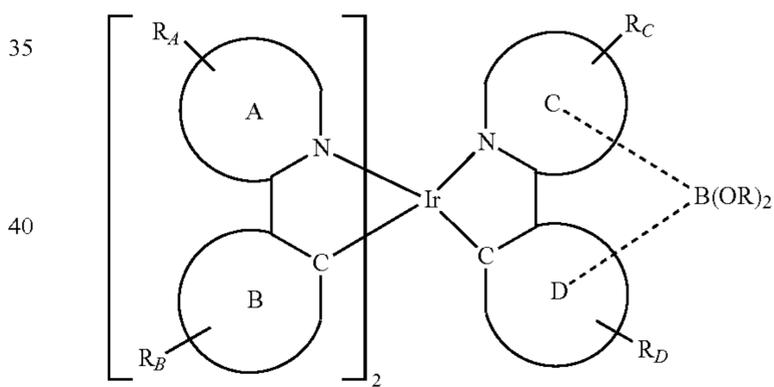
Additionally, phosphorescent emissive compounds are provided. In particular, the compounds are Ir (III) heteroleptic complexes having extended conjugation on the heterocyclic ring which coordinates to the metal through nitrogen. The compounds provided have the formula selected from the group consisting of:
