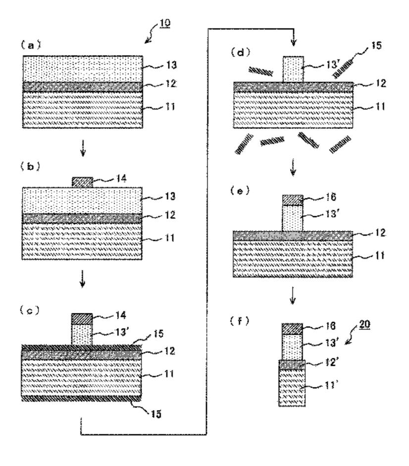
ammonium fluoride, the hydrofluoric acid in the solution mixture having a molarity of 0.5 M or more and less than 5 M.
