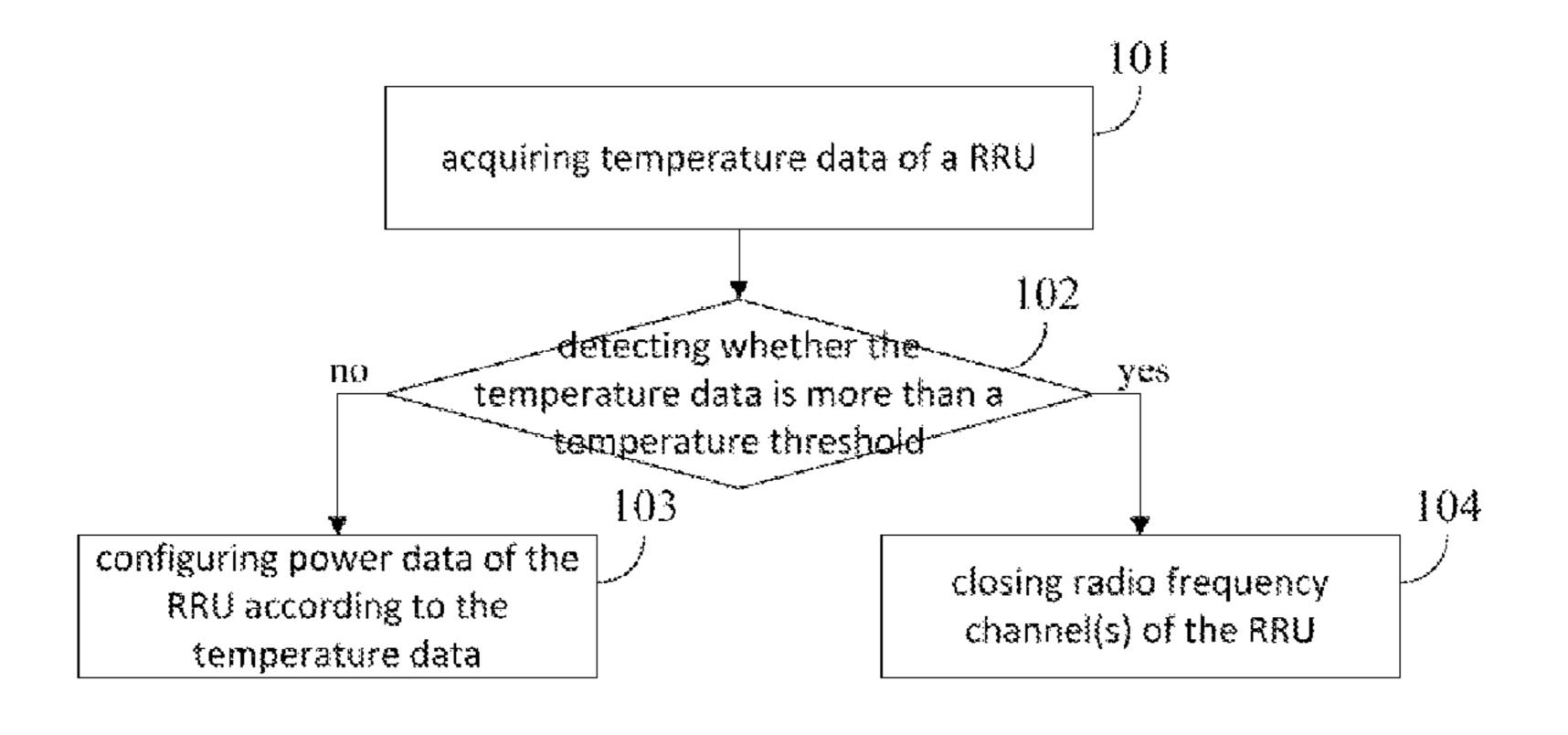
radio frequency channel(s) of the radio remote unit when the temperature data is more than the temperature threshold.
