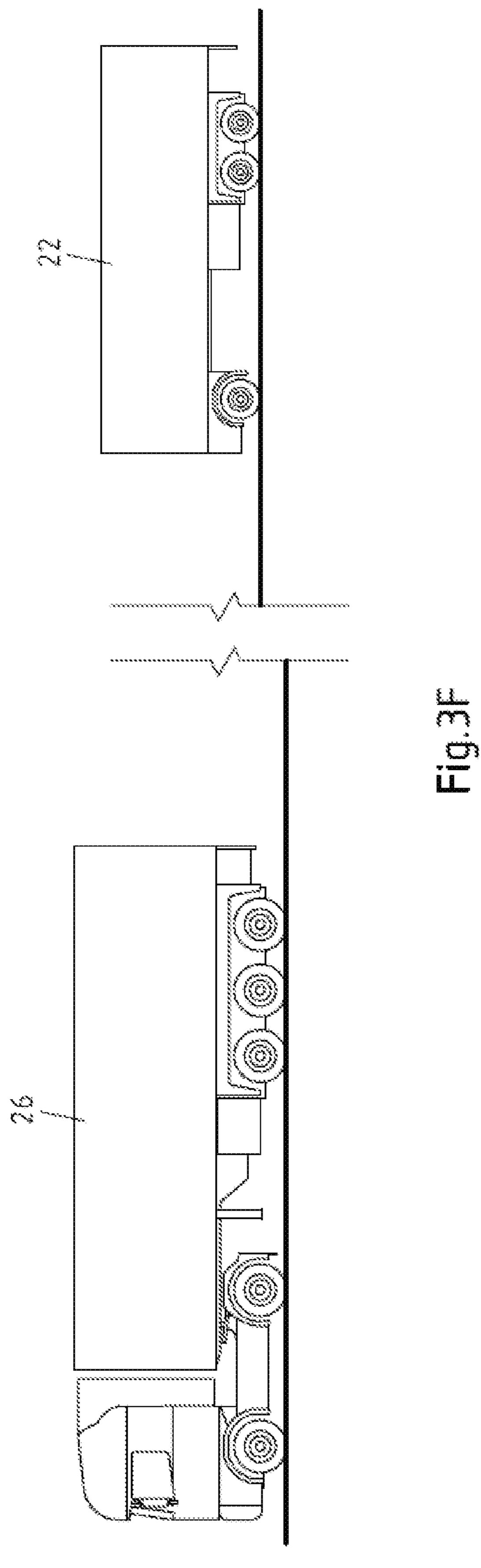
Transferring vehicle and receiving vehicle roughly approach one another on the basis of position data of the transferring vehicle and/or of the receiving vehicle
