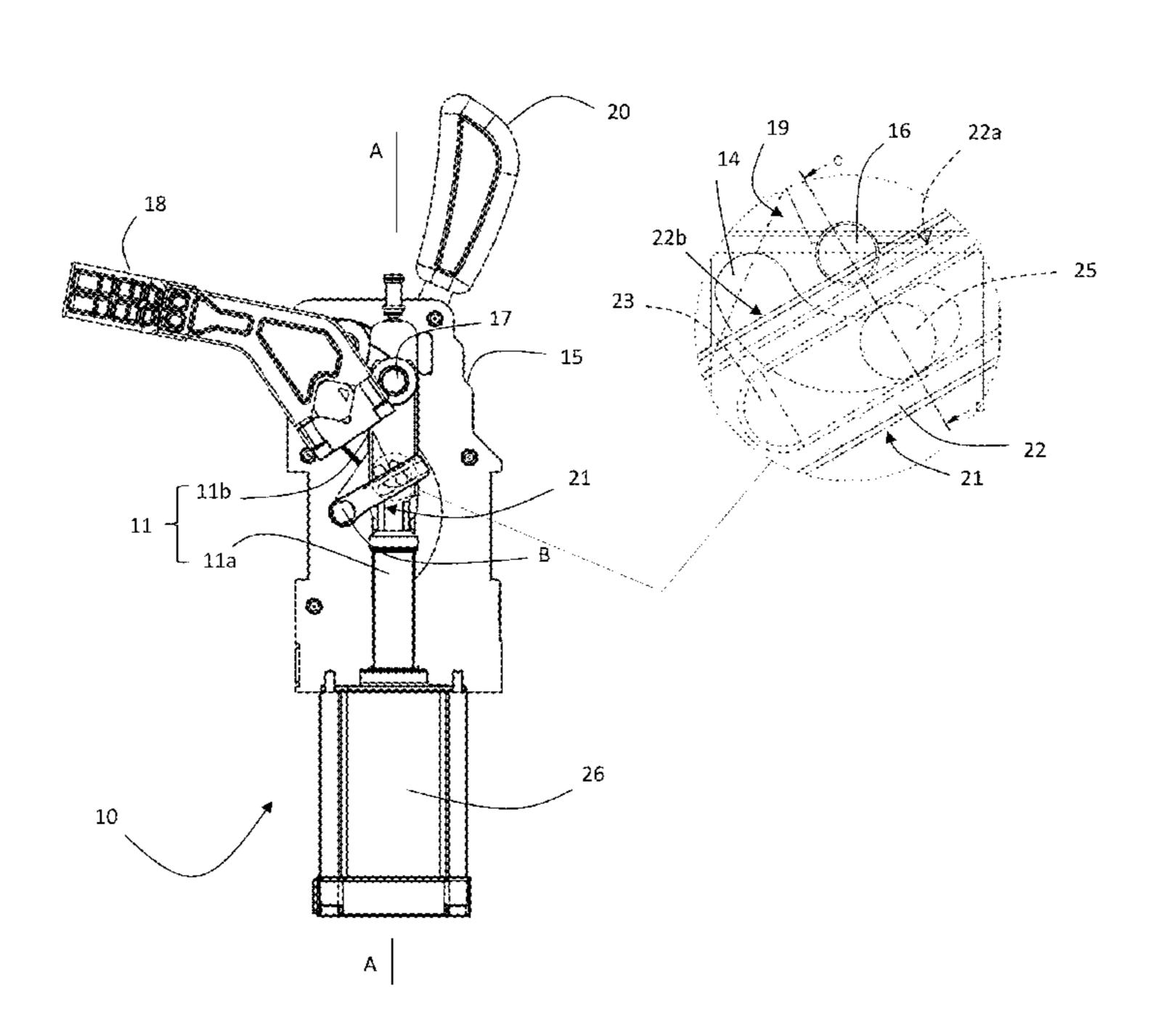
rotation of the manual operating element; the linkage comprising at least one lever arm coupled to a respective driver member, wherein the driver member is guided and constrained into a respective blind seat provided on the actuating element, characterized in that the lever arm is slidably coupled to the driver member and the driver member is movably constrained into the blind seat.
