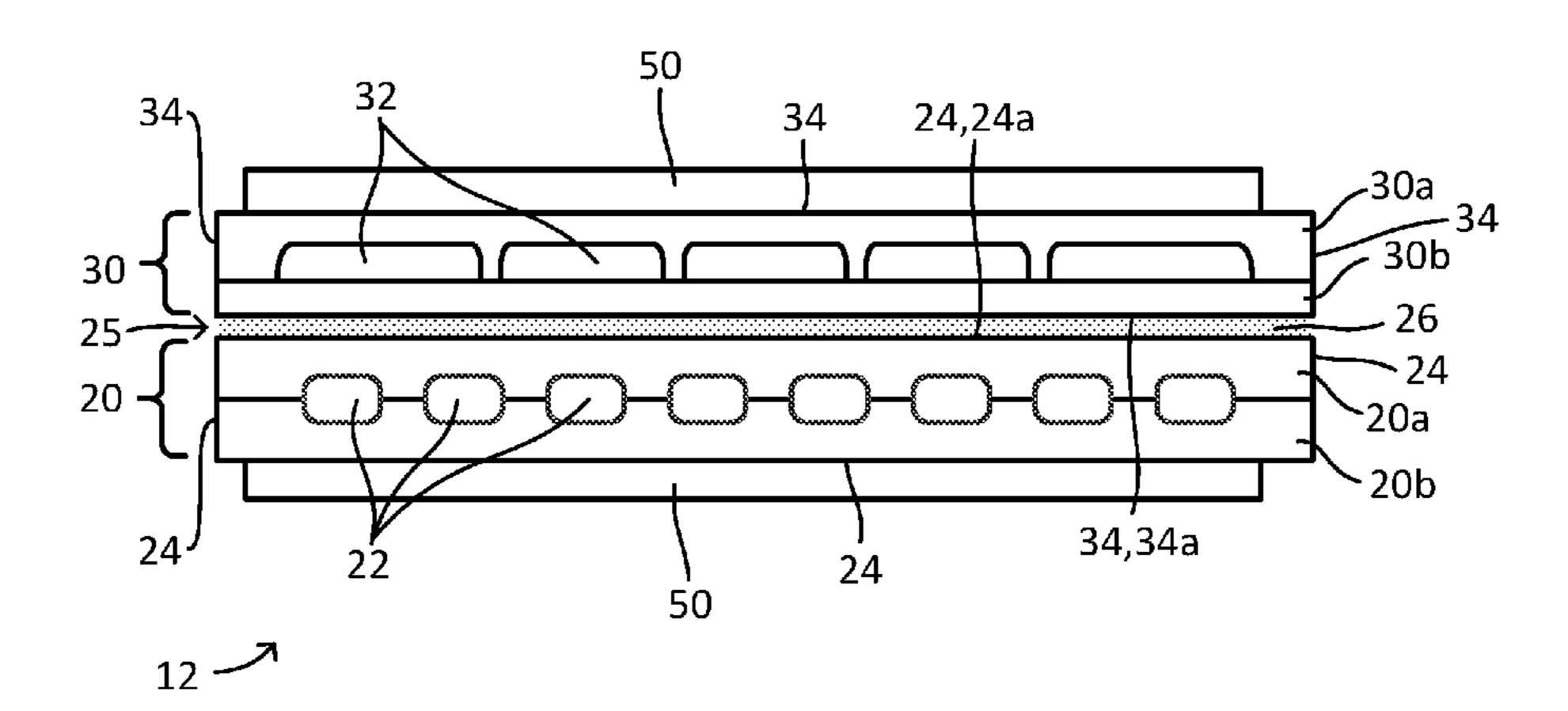
an interchangeable or replaceable substance or sheet (26) having a thermal resistance G across the gap (25), wherein G is not equal to R.
