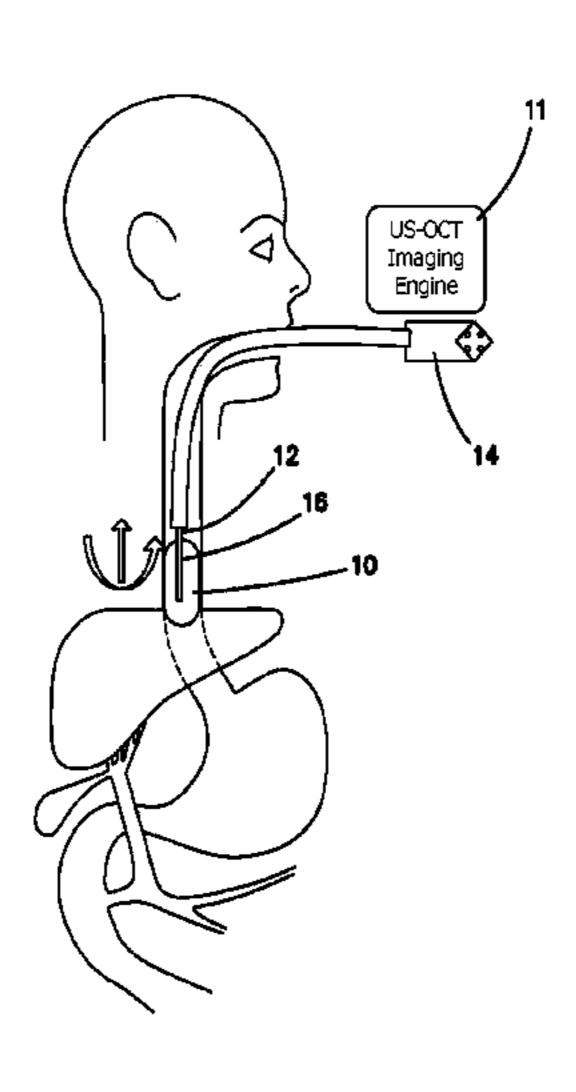
imaging and florescence subsystem for imaging. The instrumentality takes a tissue biopsy from a visible location simultaneously with the visualization of the tissue about to be biopsied so that the tissue biopsy location is visualized before, during and after the biopsy.
