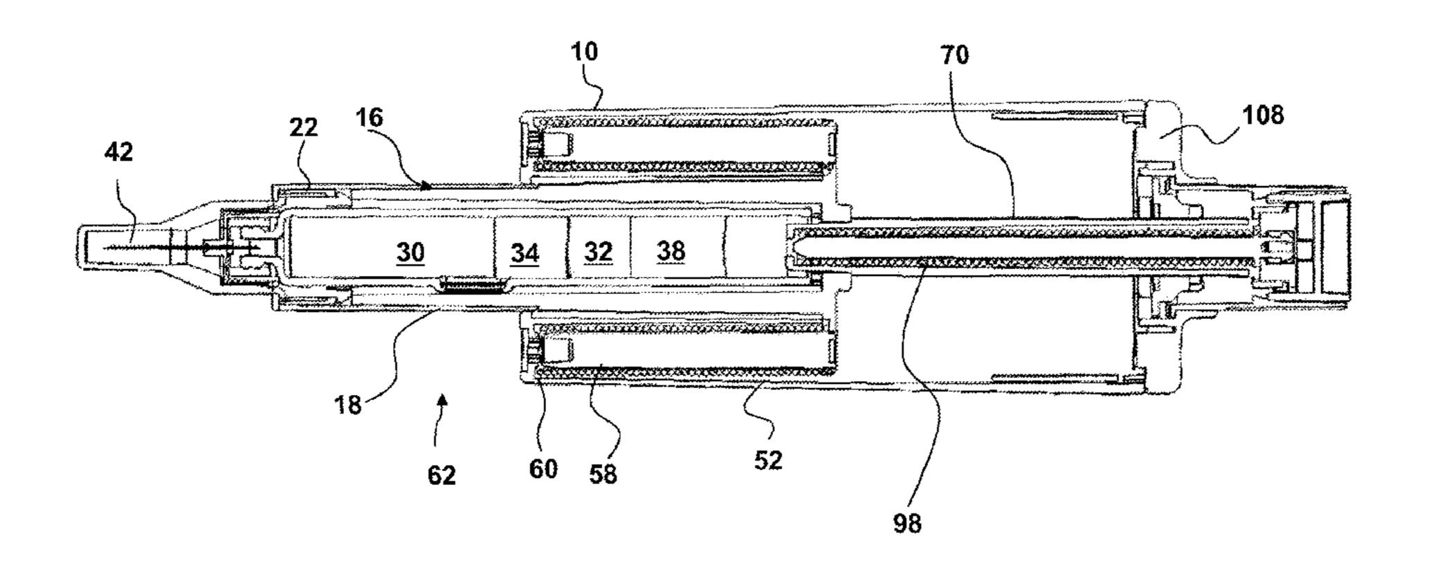
plunger rod acts on the medicament container for mixing the medicament and the diluent.
