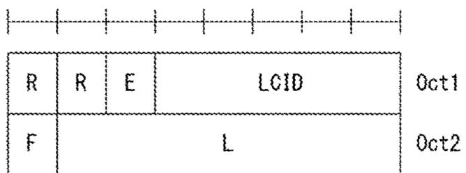
(a) R/R/E/LCID/F/L sub-header with 7-bit L field
