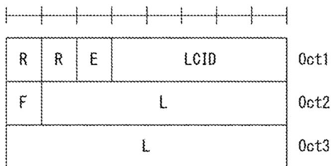
(b) R/R/E/LCID/F/L sub-header with 15-bit L field
