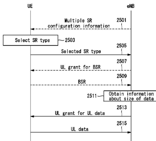
transmitting, by the UE, uplink data to the eNB through a physical uplink shared channel (PUSCH) resource allocated by the uplink grant.
