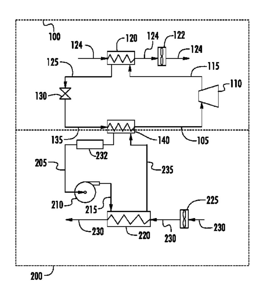
loop through the heat exchanger evaporator/condenser, including a heat rejection side of the heat exchanger evaporator/condenser, a liquid pump, a liquid refrigerant reservoir located upstream of the liquid pump and downstream of the heat exchanger evaporator/condenser, and a heat exchanger evaporator. A second conduit in a closed fluid circulation loop circulates a second heat transfer fluid therethrough having an ASHRAE Class A toxicity and a Class 1 or 2L flammability rating.
