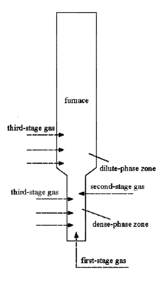
includes: blowing in a first-stage gas containing oxygen and recycled flue gas from the bottom of the furnace; blowing in a second-stage gas containing recycled flue gas from a transition zone between a dense-phase zone and a dilute-phase zone of the furnace; and blowing in a third-stage gas containing oxygen from a side wall of the furnace.
