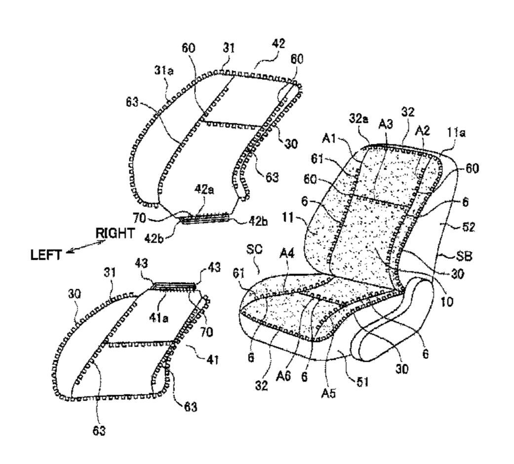
from a seated person occurs, and the inclined pile (70) of the end of the surface cover (4) is inclined in the direction in which the load resulting from a seated person occurs.
