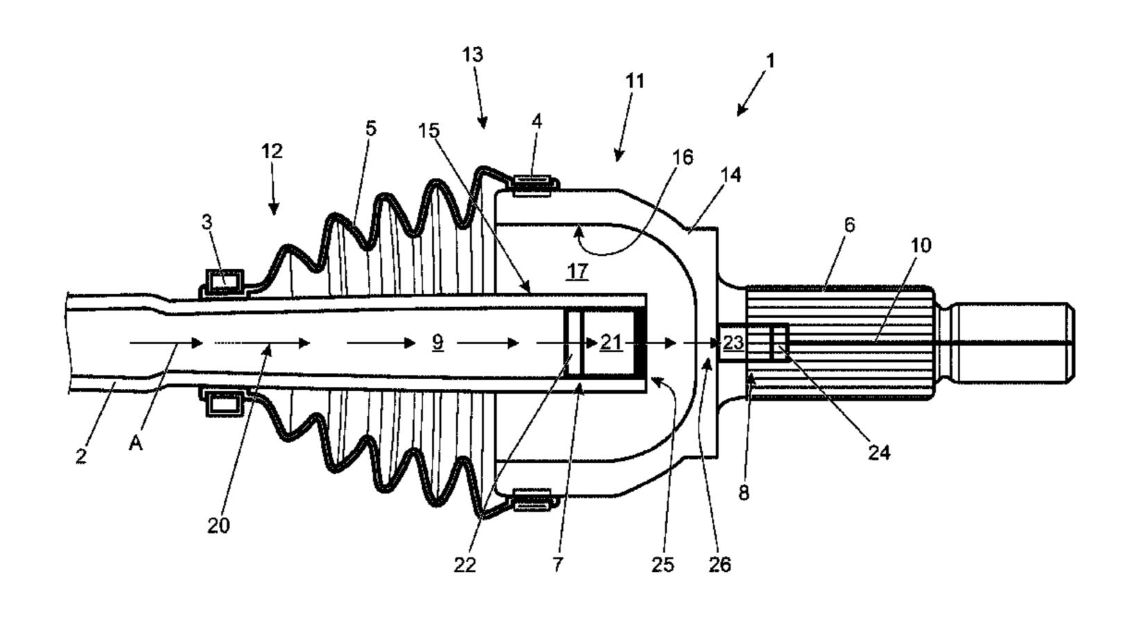
hollow driveshaft and a hollow wheel stub axle forming a CV joint having a compressed air supply line which passes therethrough. Compressed air can be supplied via the air supply line without the need for an additional fluid transfer device fluidly connecting the driveshaft and the stub axle's conduits.
