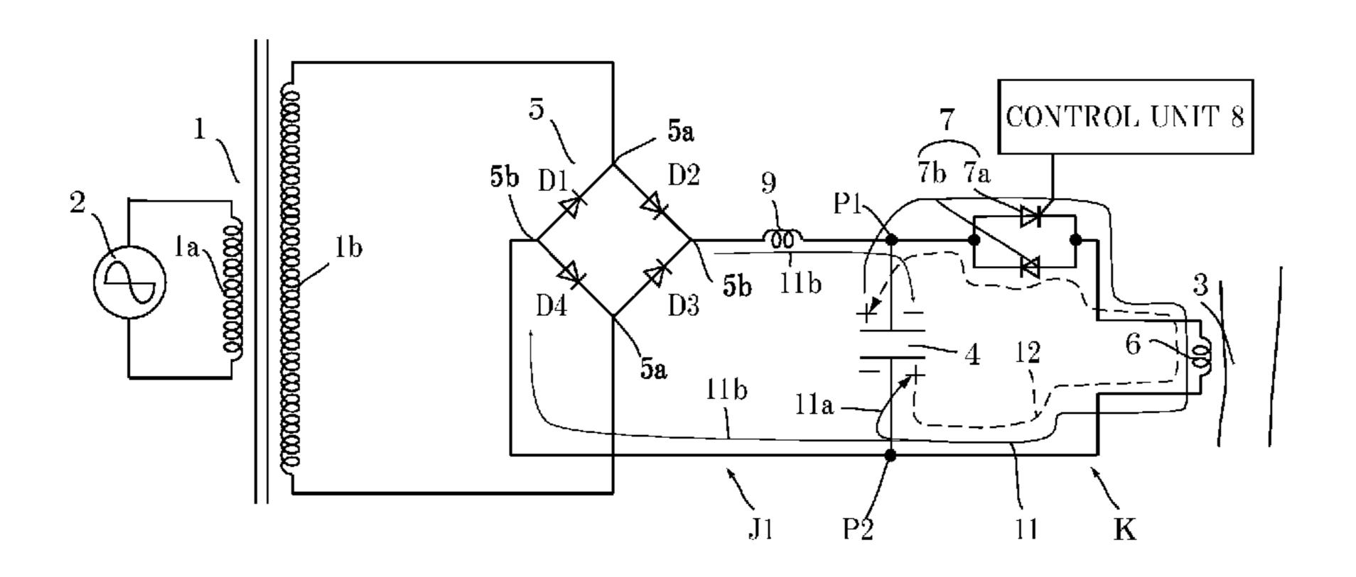
element 7 and controls conduction timing of the switching semiconductor element 7. The full-wave rectifying circuit 5 has output terminals 5b connected to both terminals P1 and P2 of the charging/discharging capacitor 4, respectively. An inductor 9 is connected between the output terminal 5b of the full-wave rectifying circuit 5 and the terminal P1 of the charging/discharging capacitor 4.
