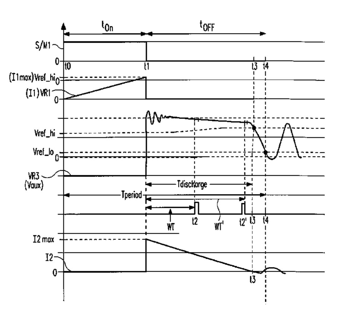
subsequent drop in the secondary current (12) to zero in order to control the secondary current (I2).
