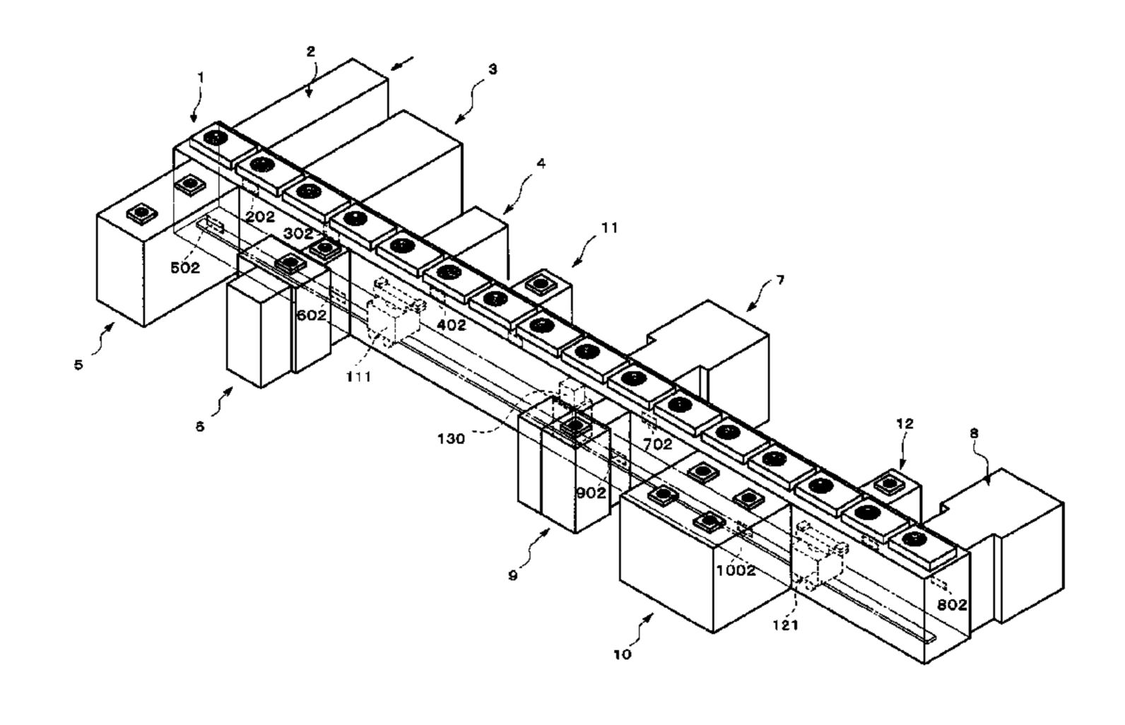
municate with each other through respective openings, and a one-way air flow in each of the openings is formed by making an adjustment such that air pressure in the transport chamber is higher than air pressure in the base material transfer areas.
