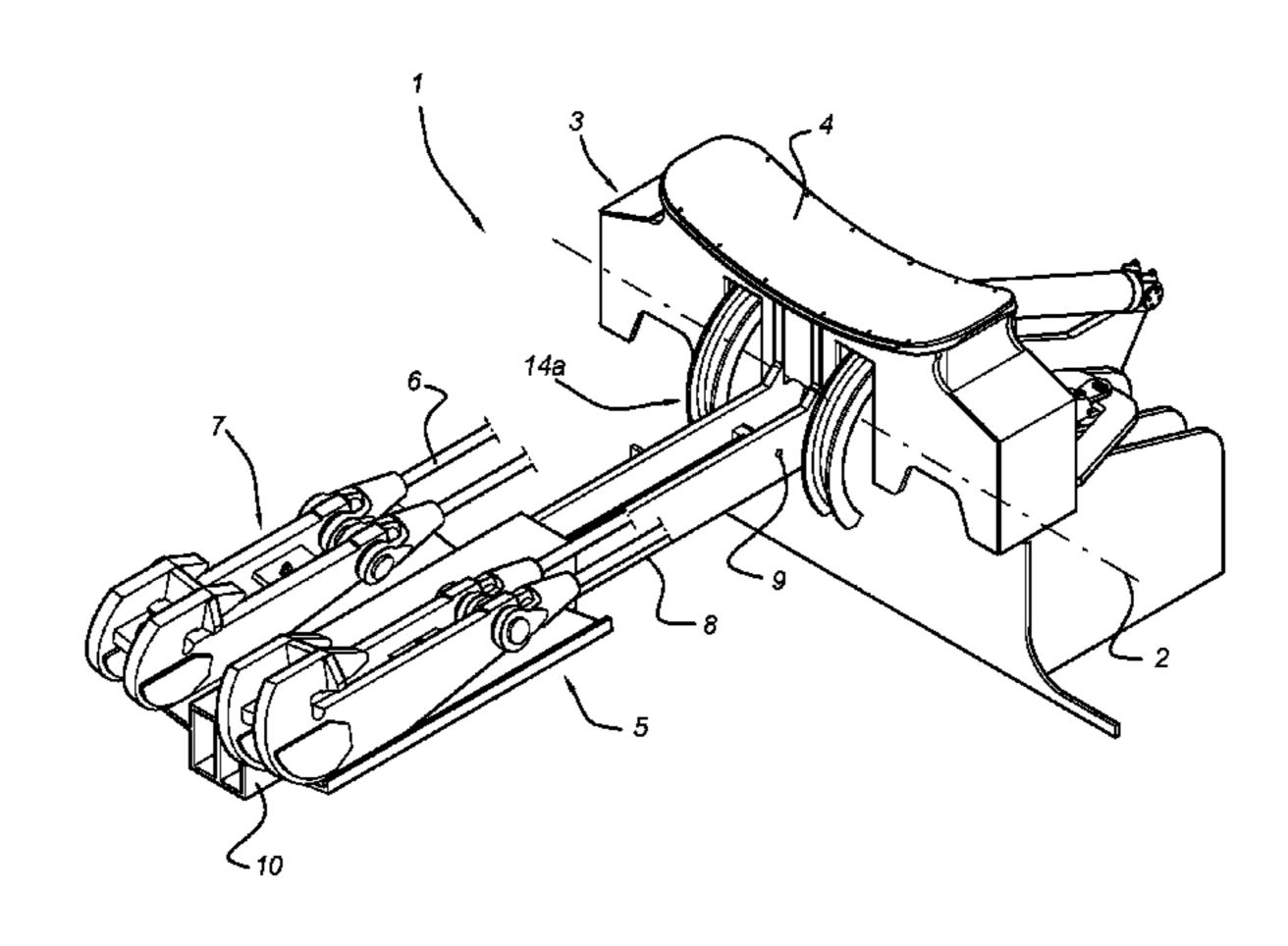
wherein the outboard support system is arranged with respect to the pile support frame such that the frame member extends transverse with respect to the support frame axis of rotation for arranging the hoisting member at a distance from the seat and aligned with the seat such that a pile may engage the hoisting member upon longitudinal movement of the pile along the seat.
