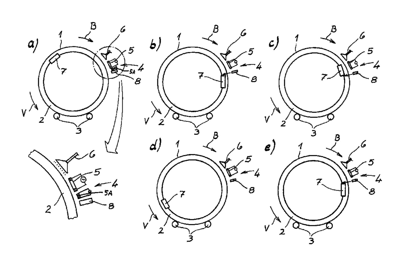
means of the sensor and the hardening device is then deactivated. The invention also relates to an arrangement which is suitable for carrying out the method described.
