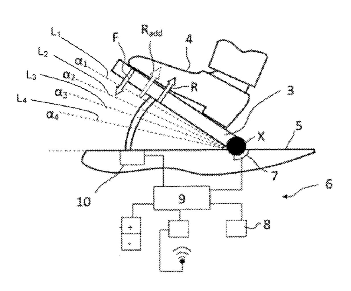
depression of the accelerator pedal reaches or is about to reach the threshold depression level; wherein at least steps a), b), and c) are automatically repeated as vehicle speed increases.
