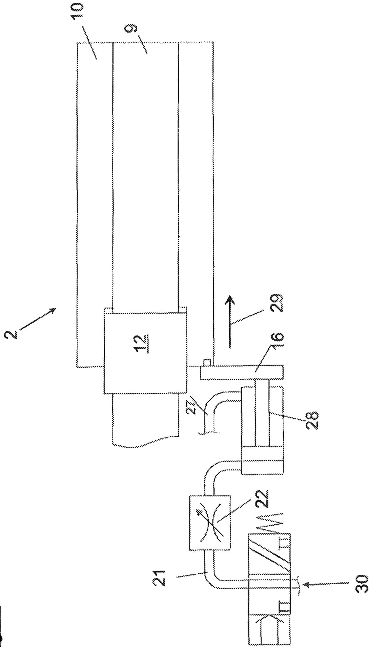
**INKING UNIT OF A PRINTING MACHINE****CROSS-REFERENCE TO RELATED APPLICATIONS**
