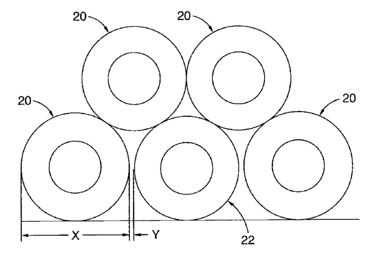
of lower layer coils in a line; the first and second predetermined ranges associated with the line in which said each coil is arranged are the same as those associated with the line in which the supporting coils are arranged.
