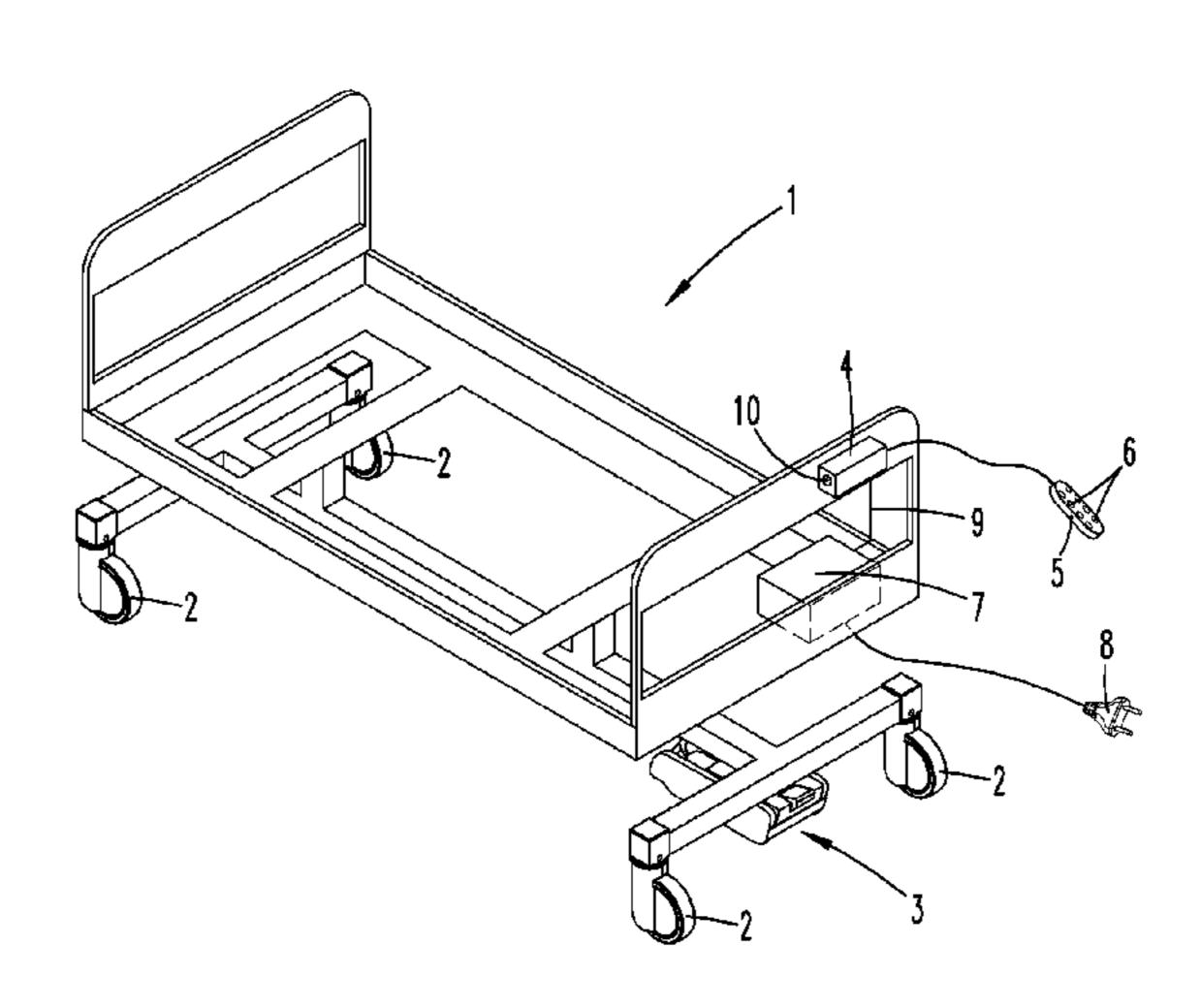
control of the rollers in combination with the additional roller and also to provide an advantageous control method for this purpose, it is proposed that the travel drive can be activated only when the rollers (2) are located in the release position or the direction-setting position.
