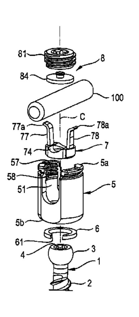
channel along the longitudinal direction in such a manner that the locking member first contacts the deformable portion and exerts a force onto the deformable portion to bring the deformable portion from the first configuration into the second configuration thereby locking the head. Thereafter the locking member comes into contact with the rod and locks the rod.
