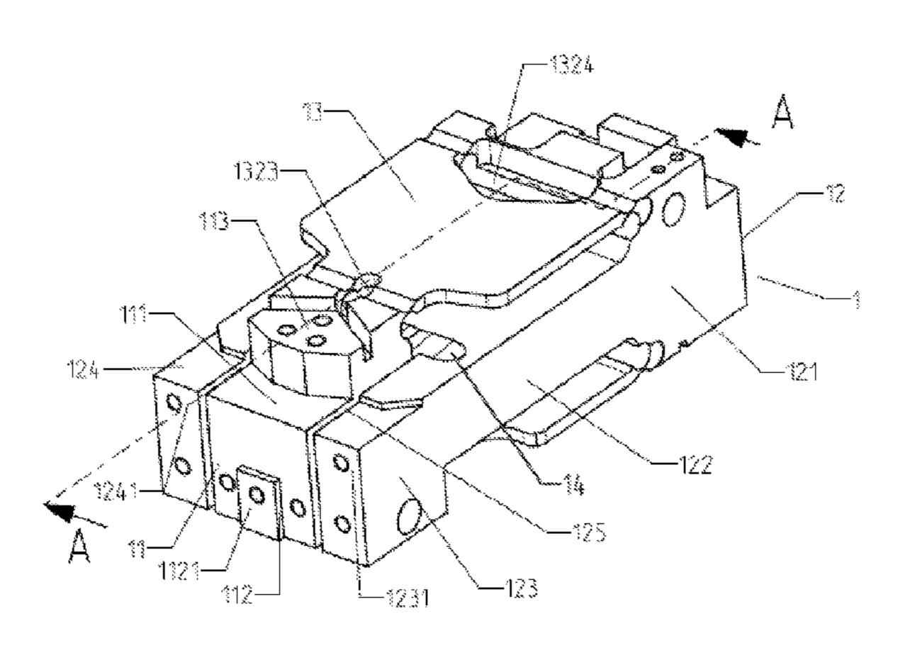
the fixing portion and the parallel-guiding members are formed integrally of one piece of solid material.
