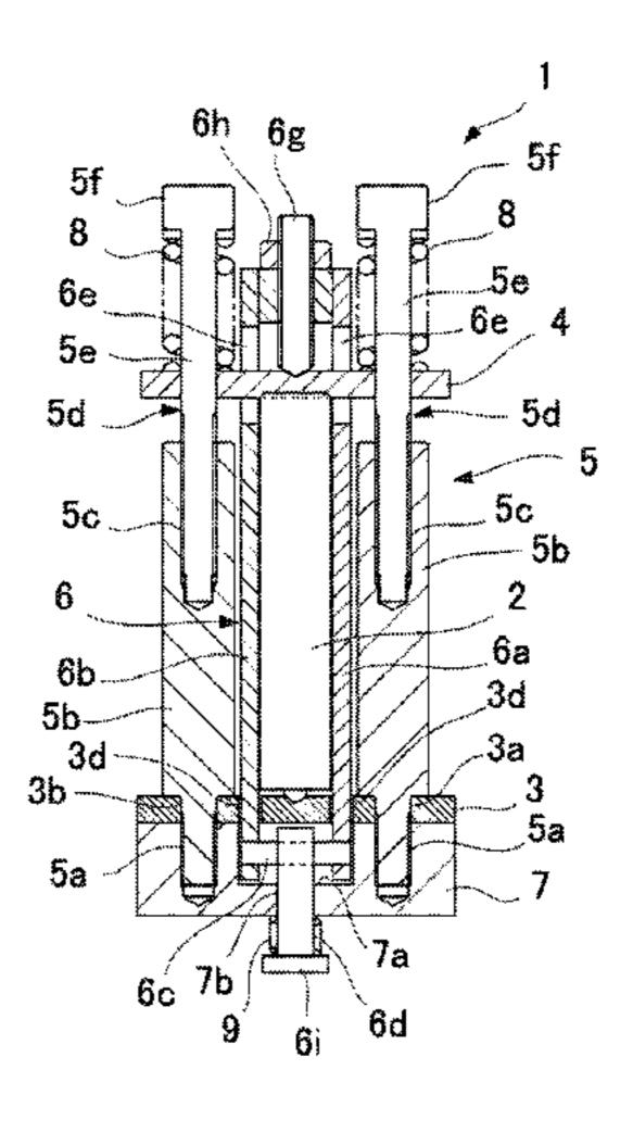
member to guide the pressing member; and a displacement transmission member which includes a pair of displacement transmission plates, an adjustment screw connected to the pair of displacement transmission plates, an output section connected to the pair of displacement transmission plates, and an elastic body that biases the output section downward.
