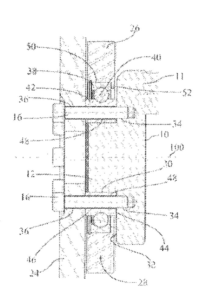
surface (30) and having a first transverse surface (44) axially bearing on the shoulder (32). The unitary guide ring comprises axial bores (48) which are aligned with the threaded holes (34) in the crankshaft and the axial bores of the flywheel (36) and have the screws (16) passing therethrough.
