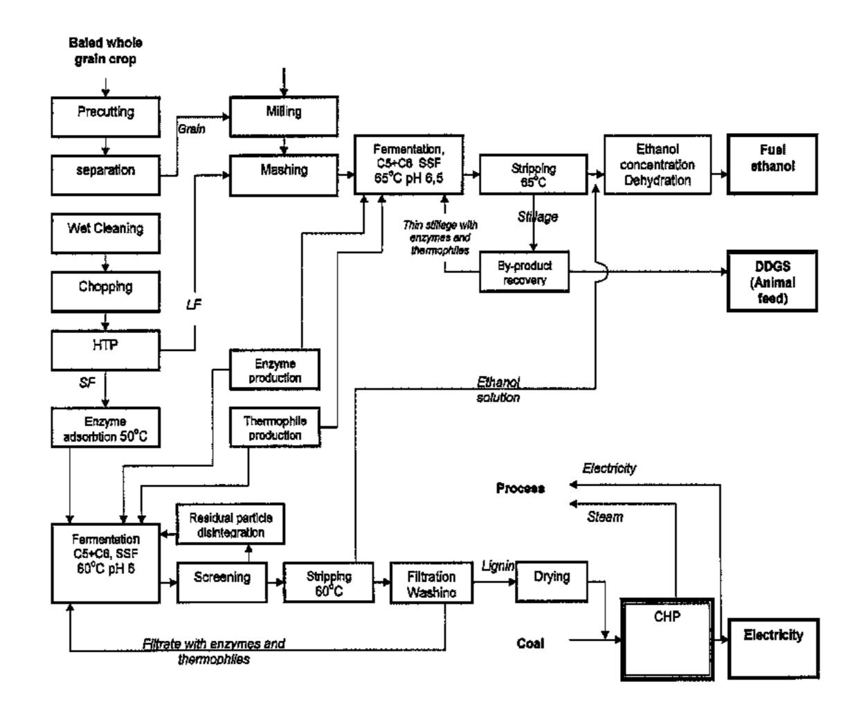
selecting the temperature and residence time for the hydrothermal pretreatment, so that the fibrous structure of the feedstock is maintained and at least 80% of the lignin is maintained in the fiber fraction.
