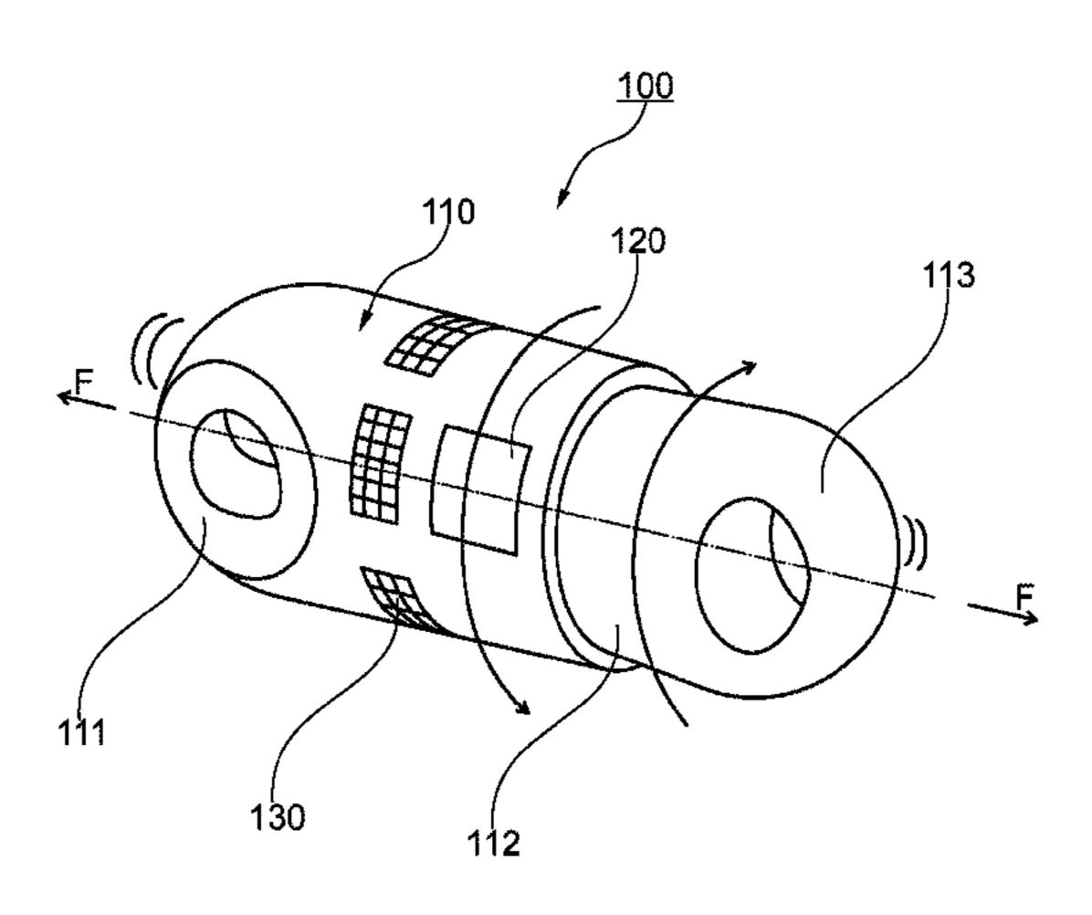
the swivel (100). A system for monitoring a mooring arrangement is also disclosed.
