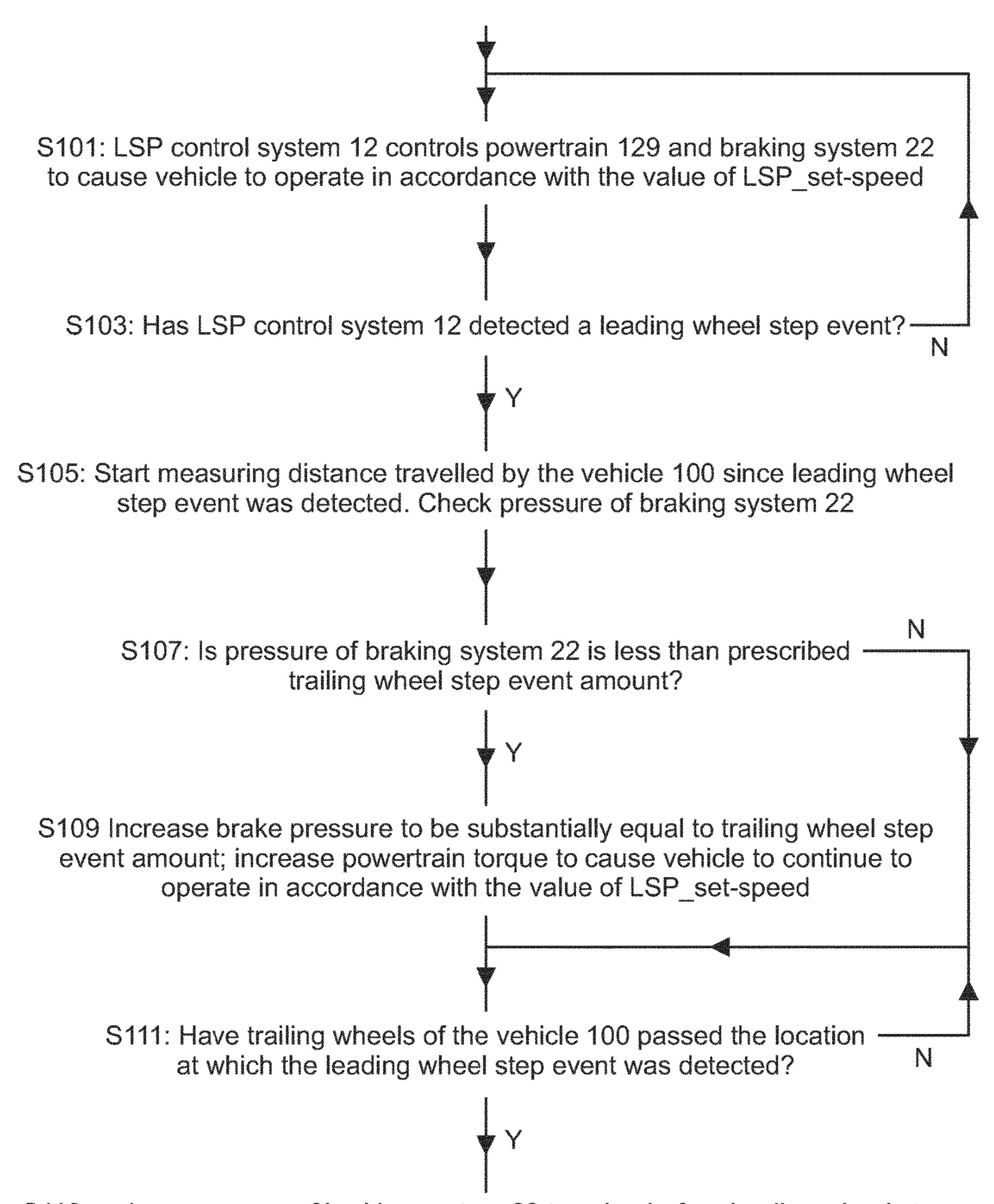
S113: reduce pressure of braking system 22 to value before leading wheel step event was detected and adjust powertrain torque accordingly
