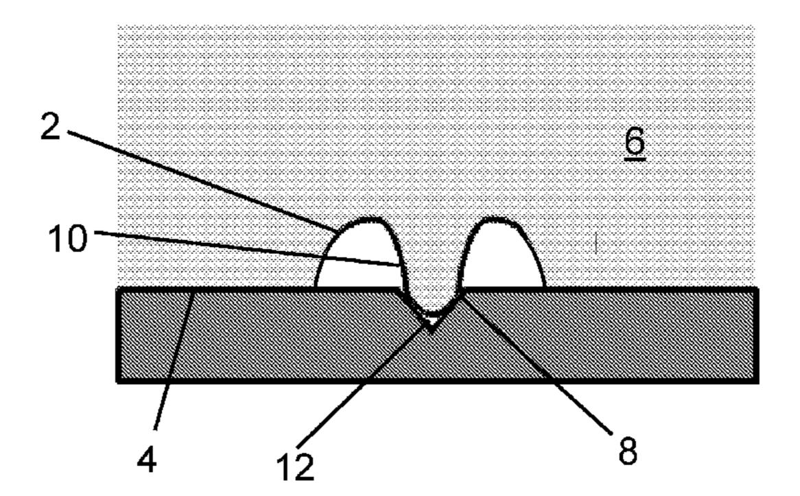
gas is trapped between the impacting jet and the surface depression. An apparatus for producing a localized concentration of energy is also provided.
