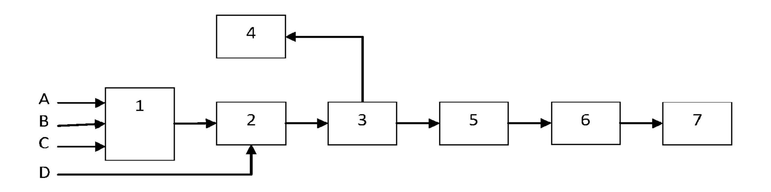
slurry, drying the coating on the electrode material by drying the organic carbonate, and surface treatment of the slurry so that the electrode is prepared for use in a lithium ion battery cell.
