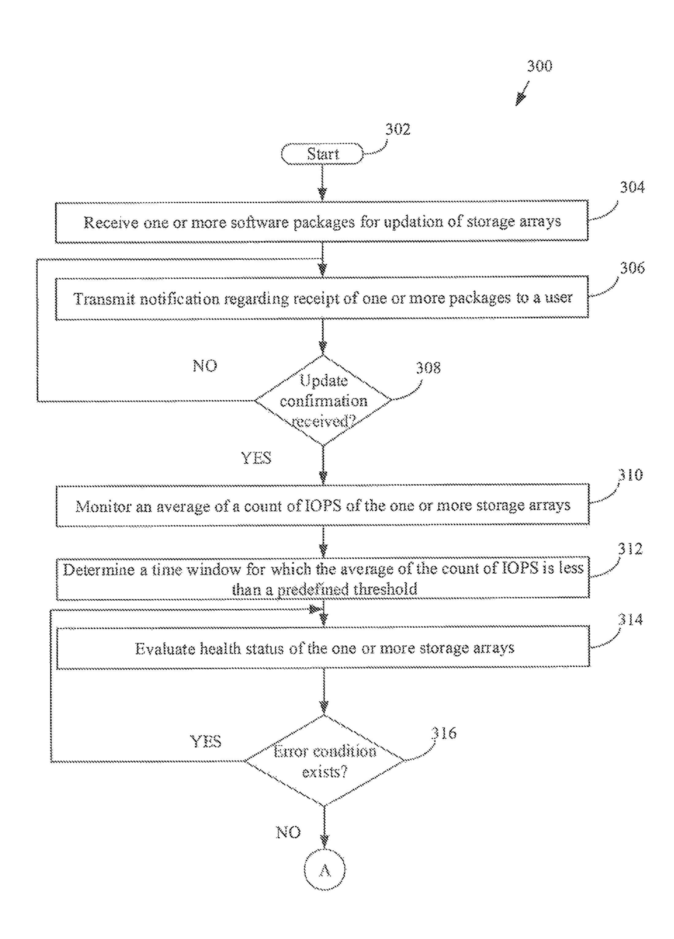
FIG. 3A: Method 300 for updating software packages in a storage system
