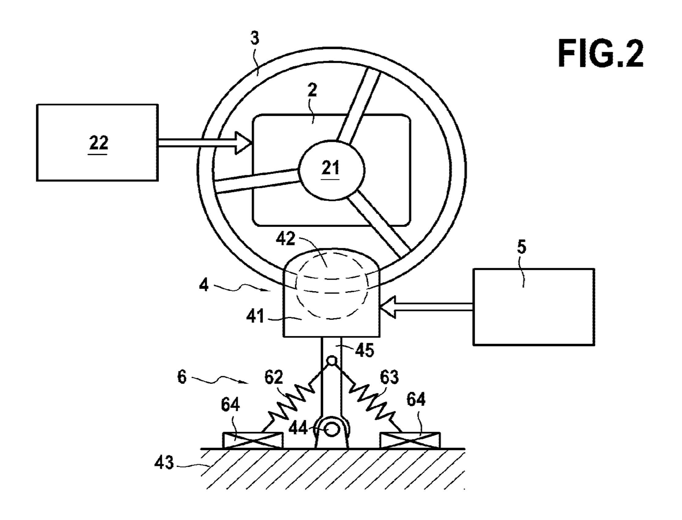
SYSTEM FOR REPRODUCING A DRY FRICTION TORQUE APPLIED TO AN ACTUATOR OF A VALVE LOCATED IN A HYDRAULIC LINE OF AN ENGINE OF A SPACECRAFT INCLUDING AN ELECTRICAL ACTUATOR CONTROLLING ORTHOGONAL FORCES OF PLATES ON A DISC TO APPLY RESISTIVE TORQUE TO A SHAFT OF THE ACTUATOR
