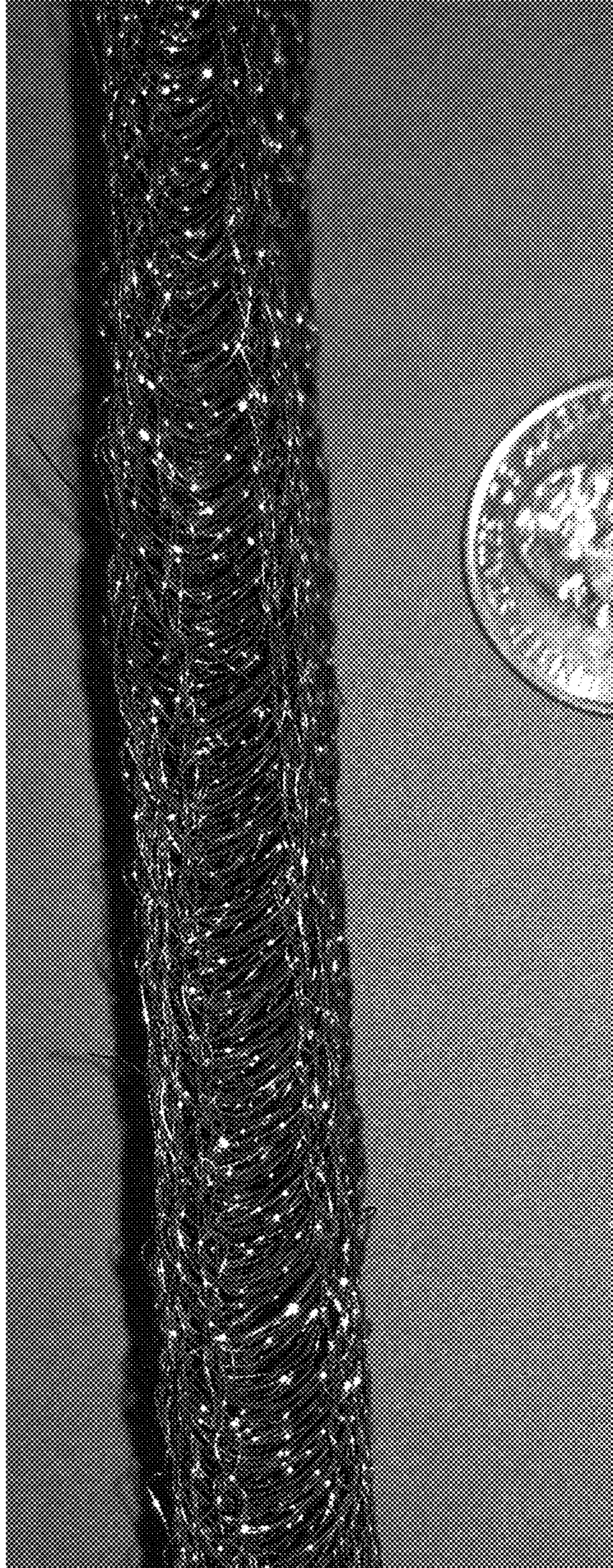
Nitinol Spacer Fabric can be knit into various height (0.750" tall)
