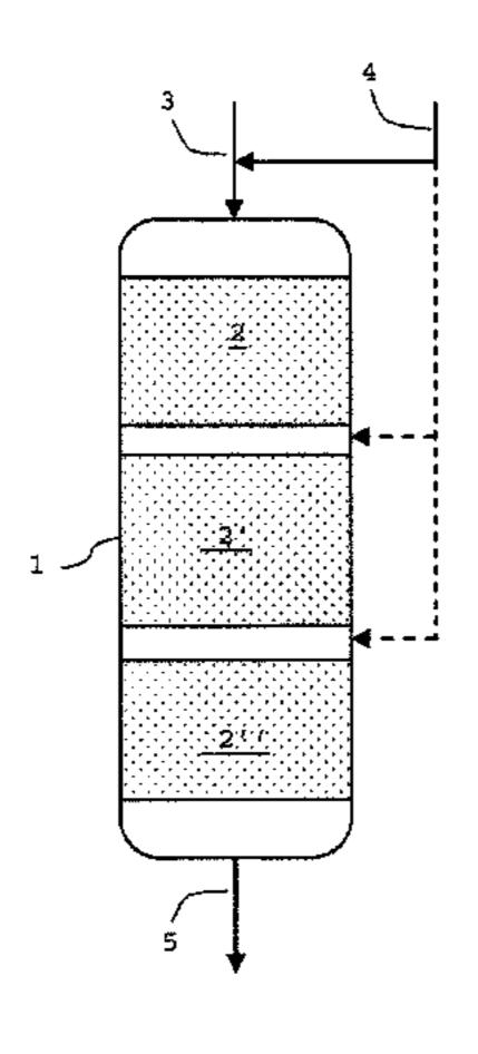
prising the step of hydroprocessing a biological feedstock using a catalyst and the step of fractionating the product of the hydroprocessing step.
