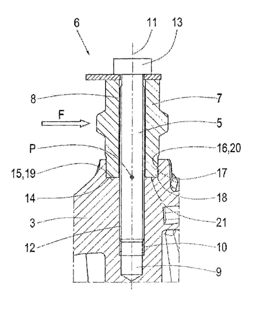
the abutment surface in such a manner that transverse forces occurring, in the radial direction in the area of the mounting, can be supported.
